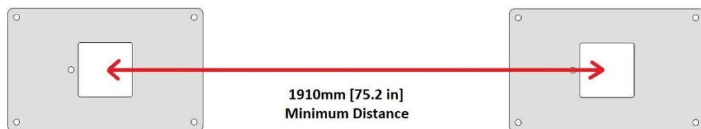
Figure 5 - 1910 mm (75.2 in.) Minimum space between pedestal baseplate centers
