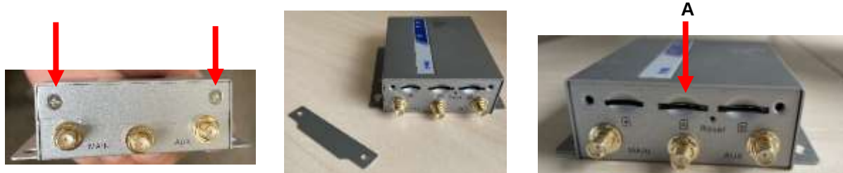
Figure 26 – For Amit Modem, remove 2 screws and slot cover to expose SIM card slots
