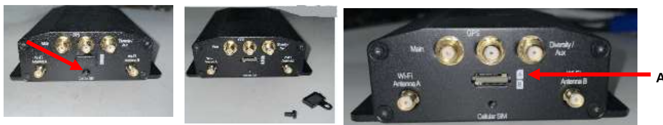
Figure 27 – For Peplink Modem, remove 1 screw and small slot cover to expose SIM card slots A and B
