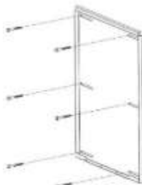
Figure 8—Lag screws and flat washers with hanging bracket
