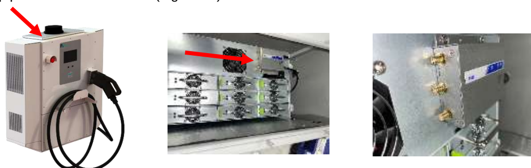
Figure 25—Remove Top Panel to access cellular modem
