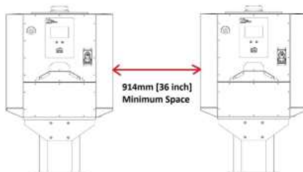
Figure 3—Minimum space between mounted chargers should be 36 in. (914 mm)
