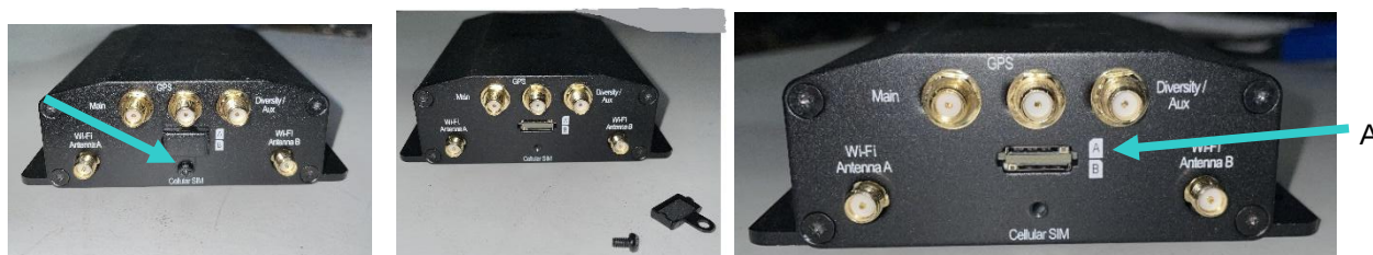
Figure 12 – For Peplink Modem, remove 1 screw and small slot cover to expose SIM card slots A and B
