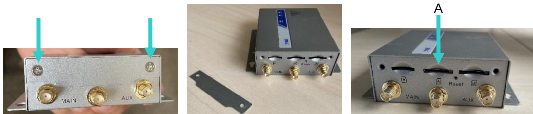
Figure 11— For Amit Modem, remove 2 screws and slot cover to expose SIM card slots
