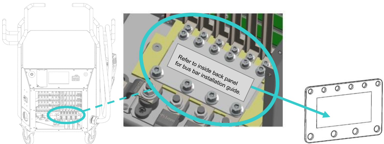
Figure 17— M6 and M8 socket head cap screws must be removed to remove plastic spacer plate
