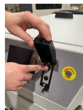
Figure 30—After entering Configuration Mode, pressing top or bottom button will increase or decrease maximum power setting
