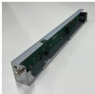
Figure 20—Install each Shelf Controller into a Shelf Controller Slot
