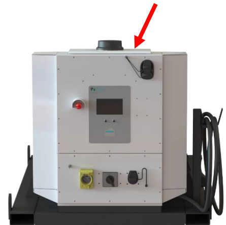
Figure 19—Remove screws around Top Panel to open
