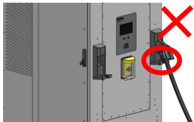
Figure 52 - Charging Cable handle not docked correctly (cable still outside holster's rubber gate)
