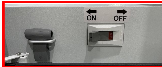
Figure 21 –Main Switch and its removeable handle shown in a fully loaded 60kW Bi-Directional Charger
